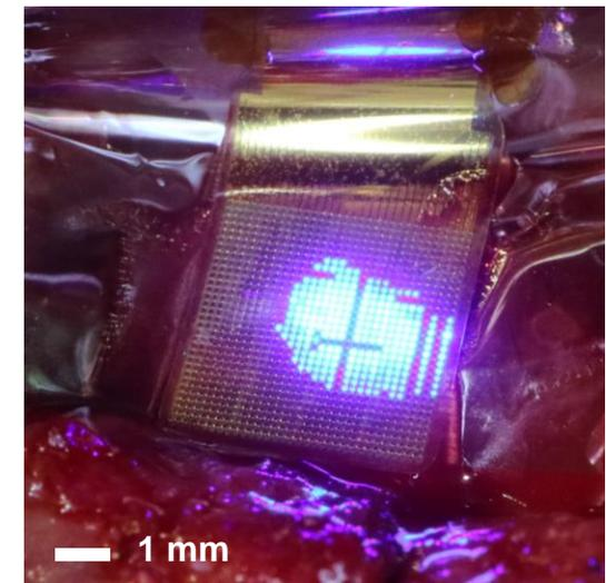
→ The sub-mm scale individual cortical column could be visualized
