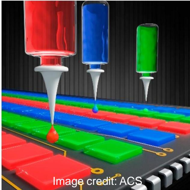
QDCC printed on micro-LEDs
