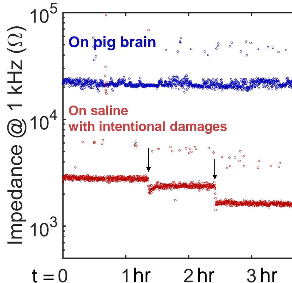
→ No electrical leakage path developed during the 3.7 hours operation on the pig brain
