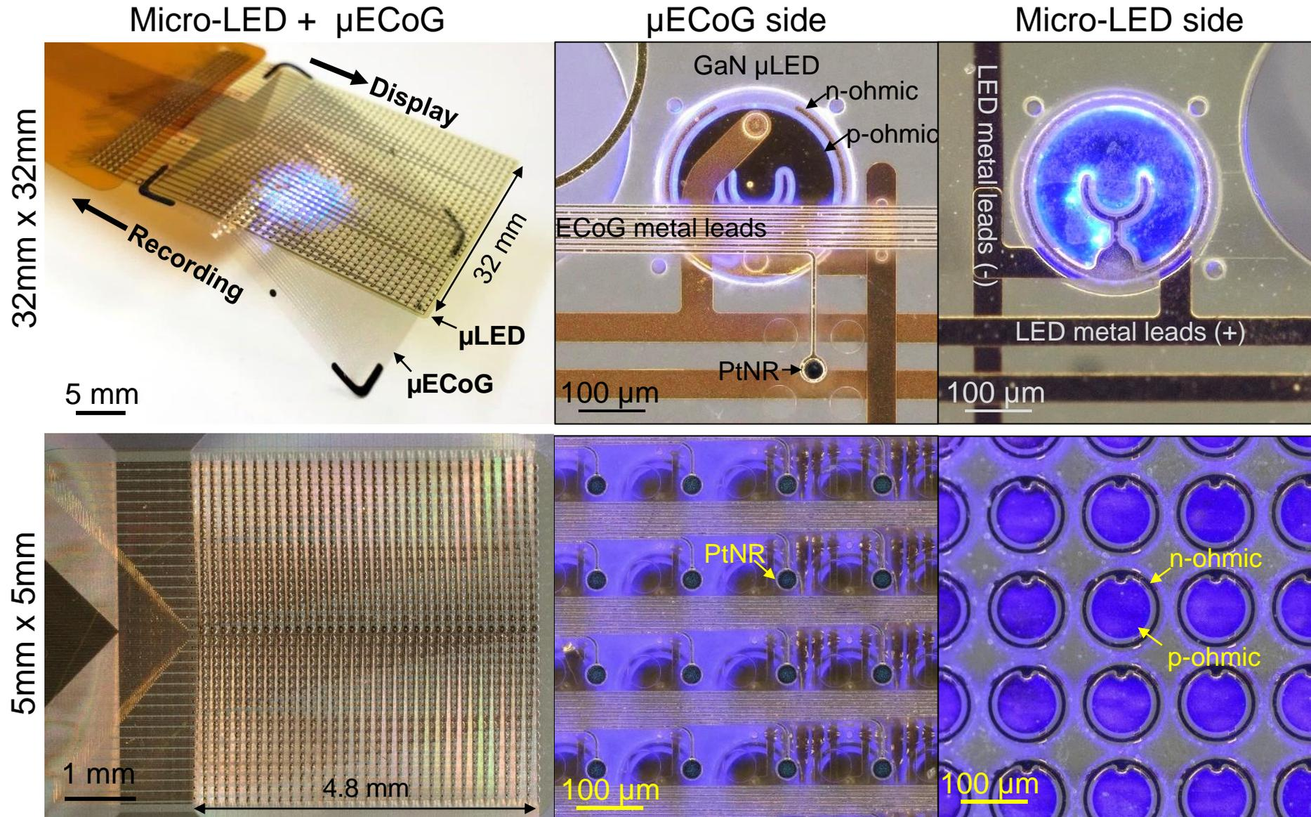
→ Flexible  $\mu$ LEDs combined with  $\mu$ ECoG grid were designed to display cortical activity
