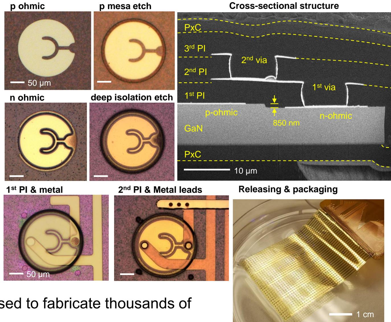
→ Scalable, monolithic process was used to fabricate thousands of micro-LED pixels on 6-inch wafers
